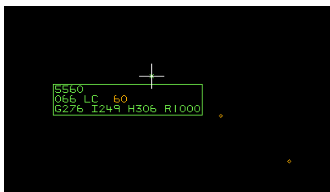
Figure 1: CPA at approximately 1920:34 – no conflicting traffic visible
