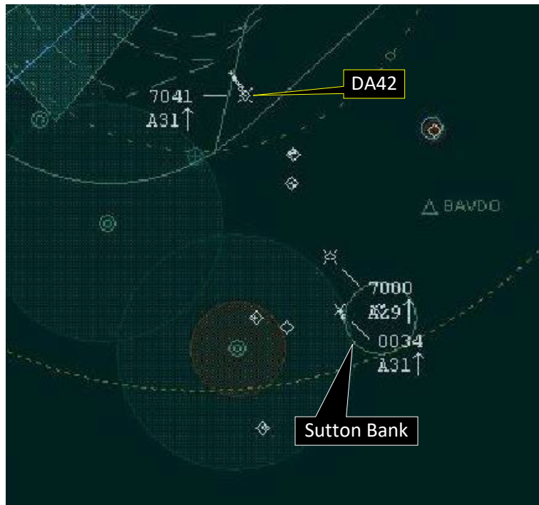
Figure 2 – Aircraft positions at 1124:10. The DA42 was observed tracking to the southeast. Traffic Information was passed to the DA42 pilot on several contacts ahead of their track.
