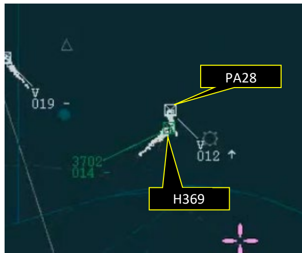
Figure 2 - 1112:20. The H369 pilot was provided additional Traffic Information on the PA28. (Separation was 0.8NM and 200ft)
