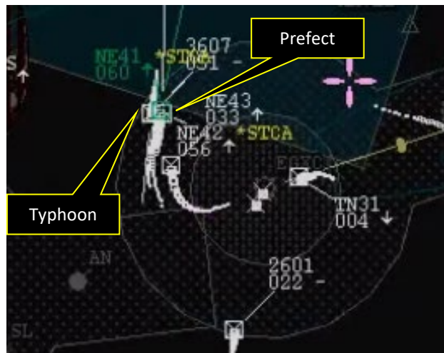
Figure 6 (1545:56): Short-Term Conflict Alert for the Coningsby Departures controller. (Separation: 0.5NM and 600ft)
