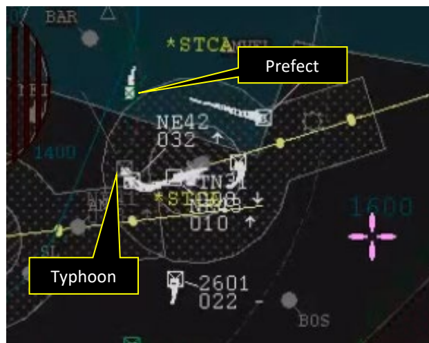
Figure 4 (1545:26): Short-Term Conflict Alert for the Waddington Lower Airspace Radar Service controller. (Separation: 4.3NM and 1400ft)
