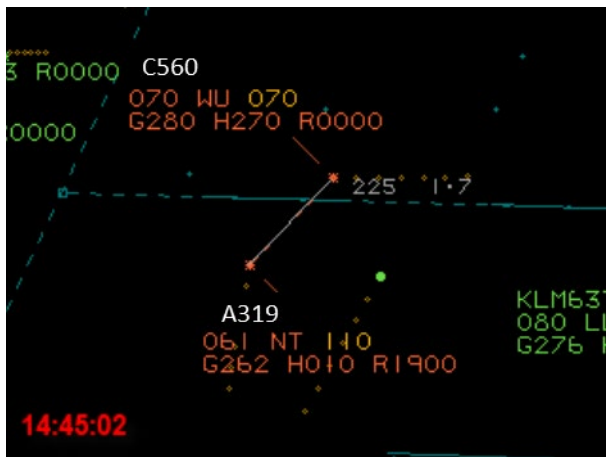
High-level Short Term Conflict Alert (STCA) activated between [A319 C/S] and [C560 C/S] at 1445:00. Separation minima between [C560 C/S] and [A319 C/S] were eroded at 1445:02. (Figure 2)
