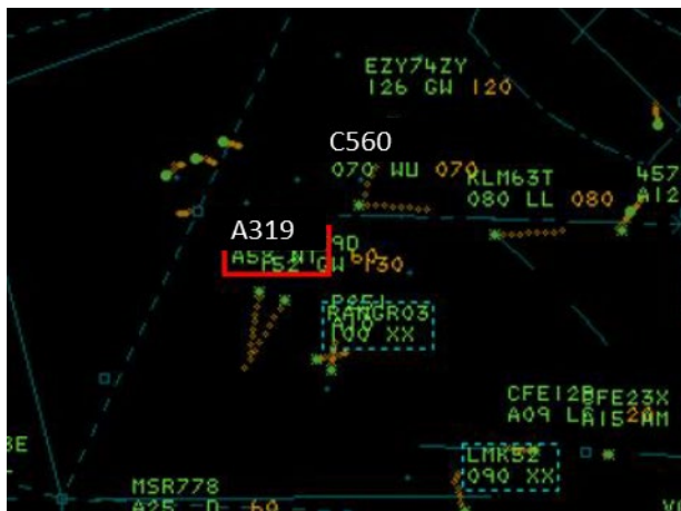
At 1444:33, the TC NW controller instructed the pilot of [A319 C/S] to climb to FL110 (Figure 1).
