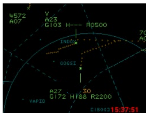
Figure 5 – Effect of [Eclipse 500 C/S] avoidance manoeuvre.
